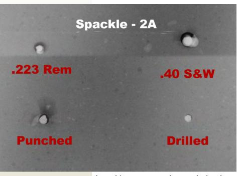
Figure 9: X-ray image of bullet holes in grid 2A, test wall 2, which were patched with spackle.
