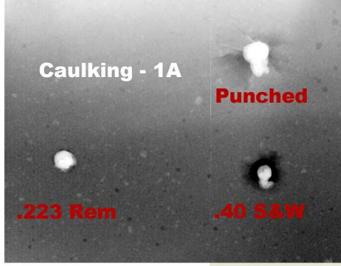
10). This air gap was the cause of the dark ring visible around the defects on the x-ray images. The x-ray image of the drilled hole showed only a thin, faint, partial ring that was clearly distinguishable from the bullet holes, likely because the hole had a uniform diameter and was more efficiently filled. The punched holes did have partial rings, but they were less distinct than the bullet holes. Though other mechanisms could result in cone-shaped defects that could also
