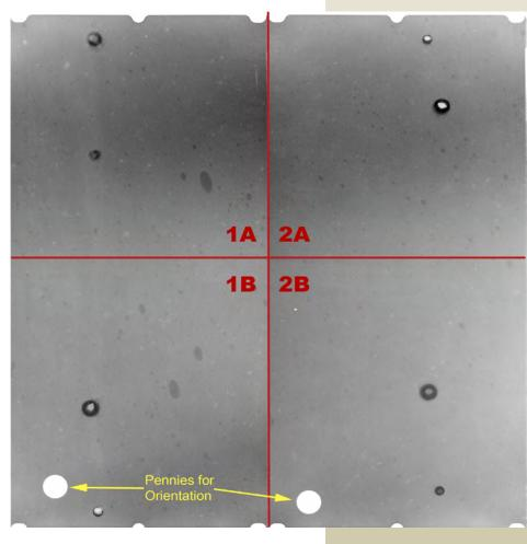
Figure 6: Plumber's putty extruded through the backside of the bullet hole during the patching process.
