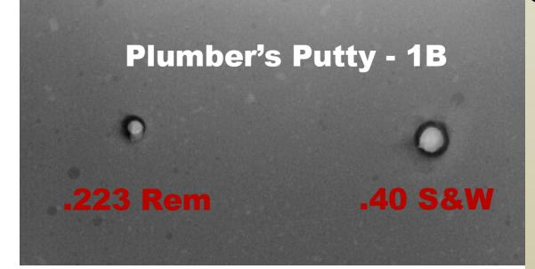
Figure 8: X-ray image of bullet holes in grid 1B, test wall 2, which were patched with plumber's putty.
