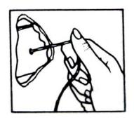
hole. Apply drywall tape around the edges, and then apply three layers of joint compound (24-hours apart), tapering wider around the hole with each layer.
