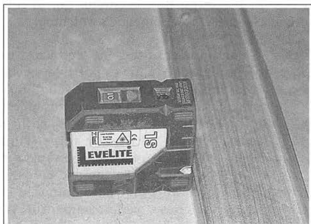
Figure 1-20. A pocket laser set up against the bottom plate of a 3\frac{5}{8} -inch wall. While the wind and vibration will affect the pocket laser to a certain extent, it’s still much faster and easier to use than a plumb bob. Use caution, though; never look directly into the beam. It can damage your eyes.
